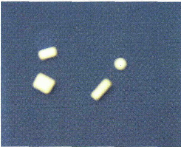
Fig. 1 Chip teflon case for TLD chip (left) and rod teflon case for TLD rod.
