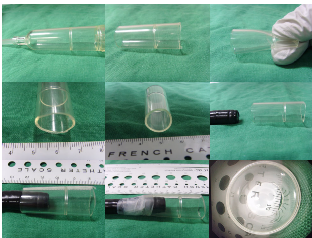
Fig. 3. modification of drip chamber of fluid set.
