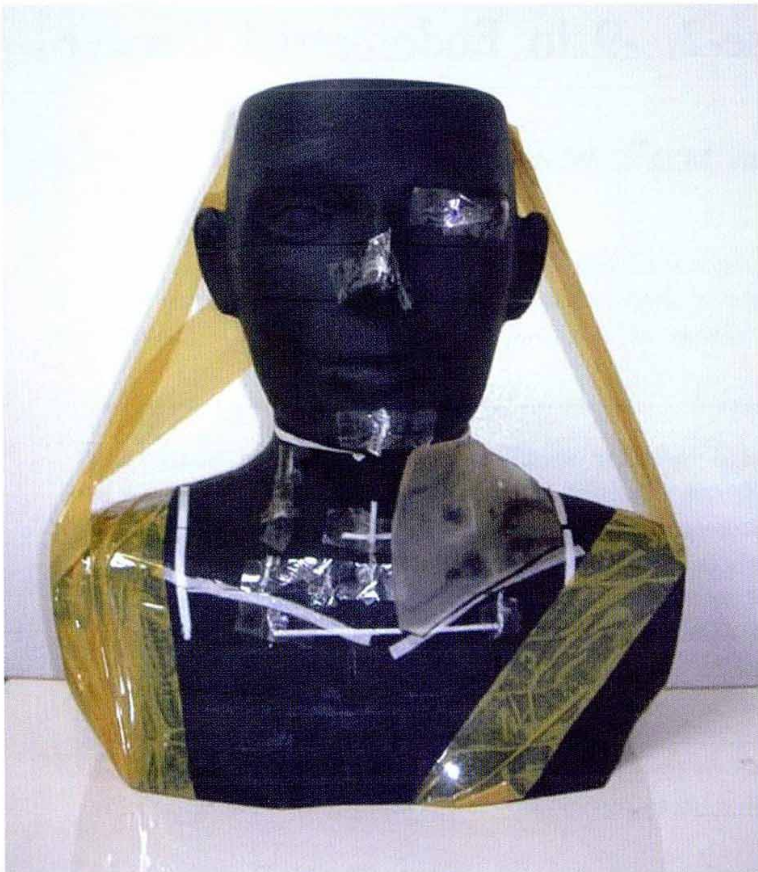
Fig. 3 Anthropomorphic phantom irradiation setup with bolus
